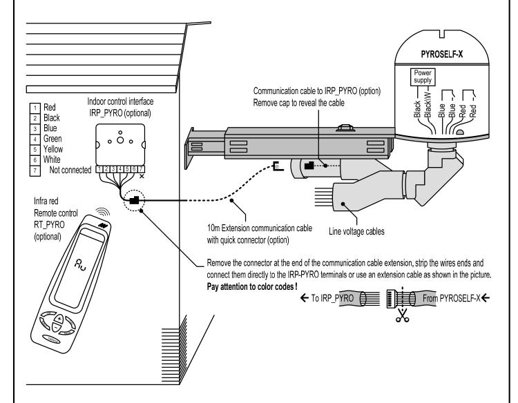
Connecting the indoor control panel IRP\_PYRO (optional):
